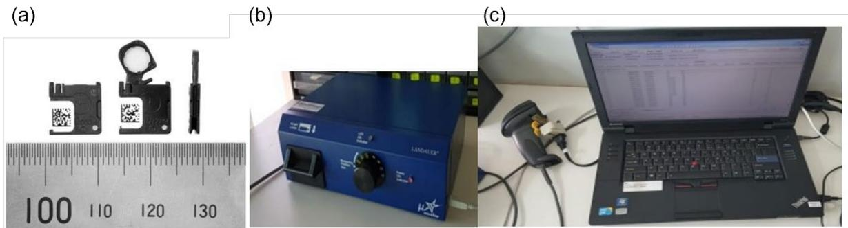
**FIGURE 1.** The OSLD dosimetry system comprising of (a) nanoDot™, (b) microStar reader, and (c) barcode reader with a processing unit
