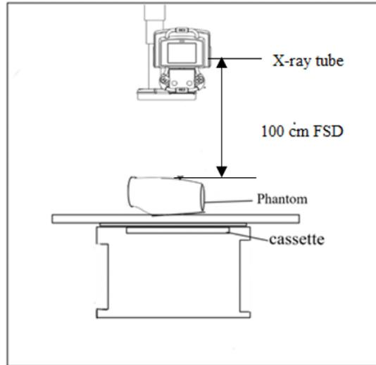
FIGURE 4: Setup position of the phantom on the X-ray table.
