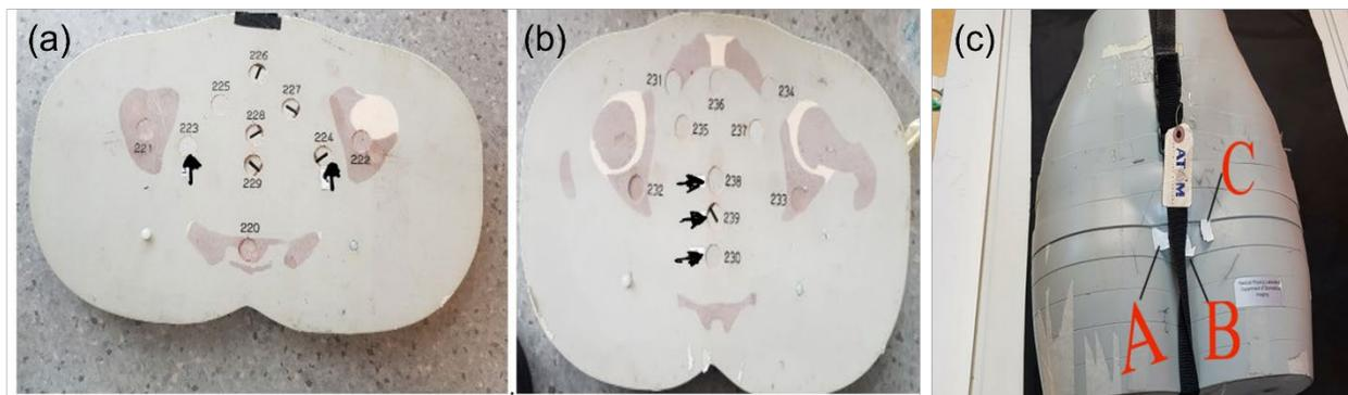
**FIGURE 2:** A cross-section of the female phantom at the (a) ovary position (b) uterus positions and for male phantom, the position representing testes at the surface of the phantom. The nanoDot™ units were placed inside the phantom at the ovary and uterus positions (indicated by the black arrows) and on the testis, indicated by the orange labels (A,B, and C).
