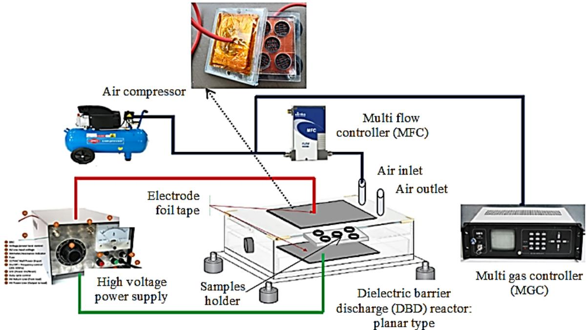
FIGURE 1. The schematic diagram of the DBD-CP system for seeds treatments.
