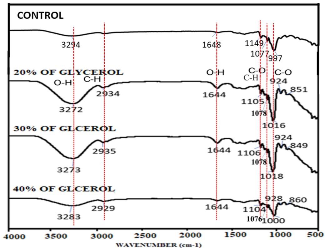
FIGURE 2. FTIR spectra for all film sample.
