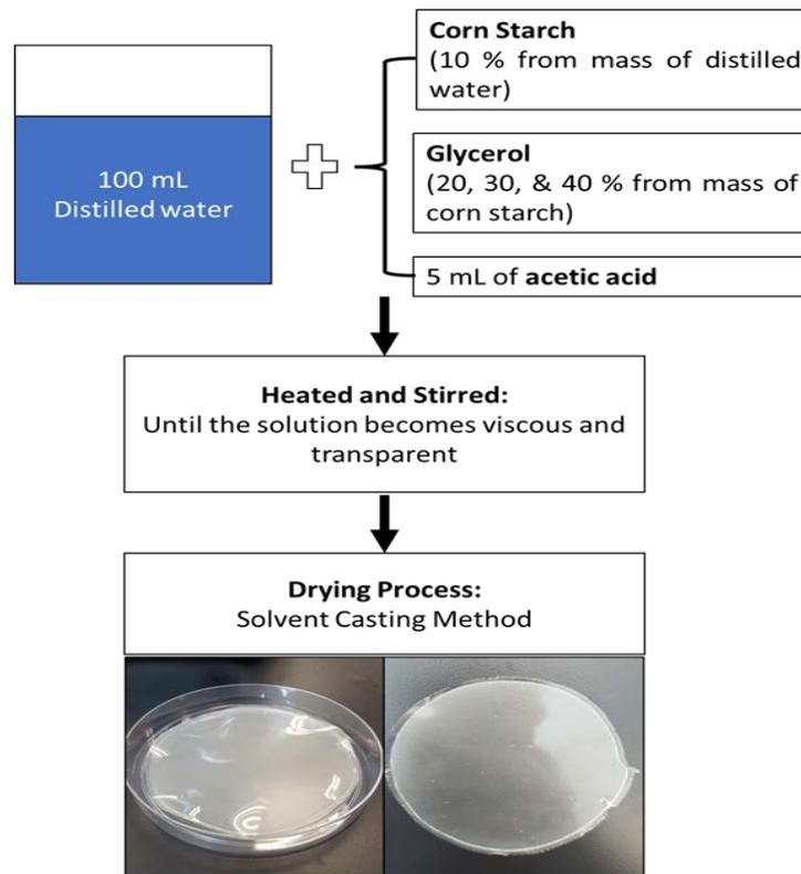
FIGURE 1. Process of making the corn-based bioplastic film.
