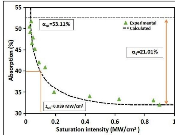
FIGURE 3. The nonlinear absorption of ITO-ZnO SA.
