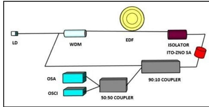
FIGURE 4. Experimental setup of passively Q-switched fiber laser.
