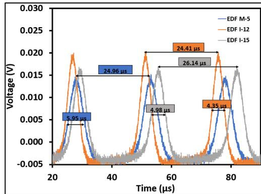
FIGURE 6. The pulse train of passively Q-switched EDFL for EDF M-5, EDF I-12 and EDF I-15.
