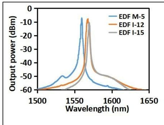
FIGURE 5. The optical spectrum for EDF M-5, EDF I-12 and EDF I-15.
