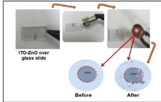
FIGURE 1. Mechanical exfoliation process.
