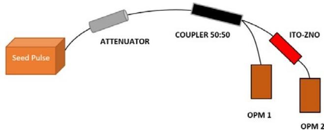
FIGURE 2. Nonlinear saturable absorption of ITO-ZnO measurement setup.
