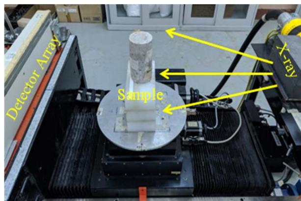
**FIGURE 3.** X-ray CT system: fan-beam, rotate only
