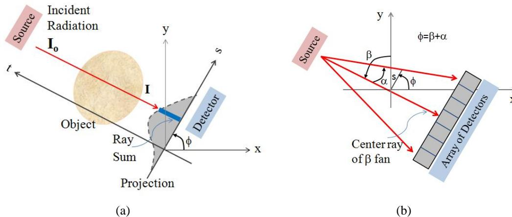
FIGURE 1. CT Data acquisition (a) Parallel beam (b) Fan beam
