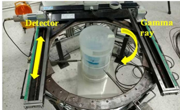
FIGURE 2. Gamma ray CT system: parallel beam, translate-rotate
