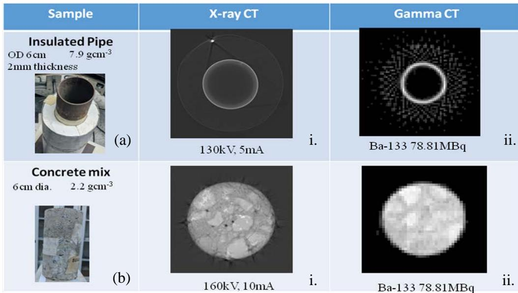
**FIGURE 4.** (a). An empty insulated pipe sample consists of mild steel, calcium silicate and aluminium jacket. Figures 4(a)i and 4(a)ii show the pipe's x-ray and gamma ray cross sectional images respectively. (b). A core sample of building concrete consists of cement and aggregates. Figures 4(b)i and 4(b)ii show the core's x-ray and gamma ray cross sectional images.
