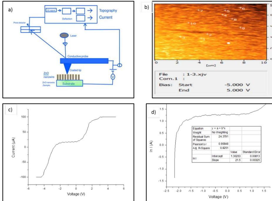
**FIGURE 2.** a) Schematic of setup C-AFM measurement b) 2-d mapping of ZnO by C-AFM c) I-V plot data of the Schottky contact (Pt/ZnO) for S5 d) Semi-log represents I-V characteristic curve.
