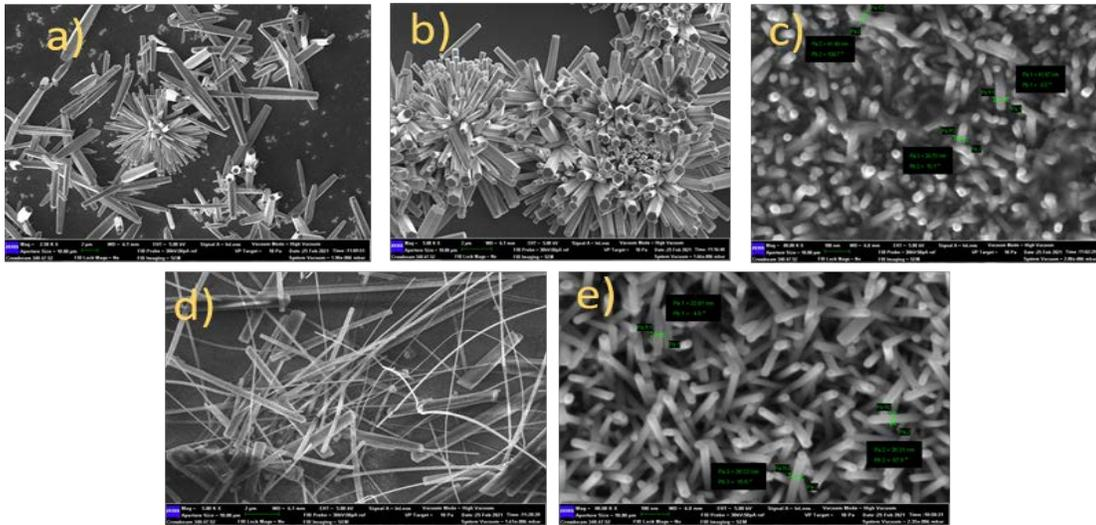
FIGURE 1. shows the Morphology of ZnO nanowire by FESEM a)S1, b)S2, c)S3, d)S4, e)S5
