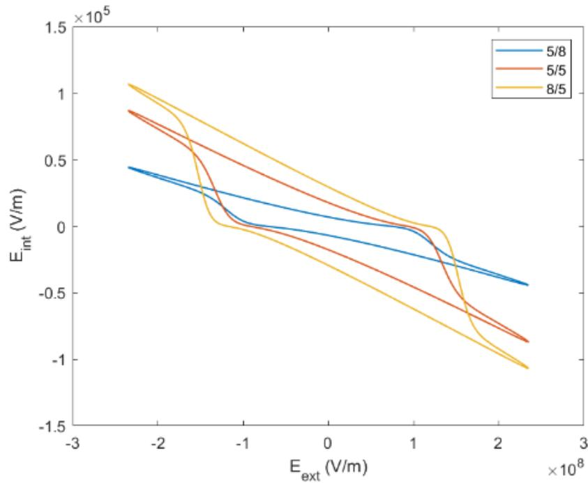
FIGURE 4. Internal electric field-applied electric field ( $E_{int} - E_{ext}$ ) hysteresis loops of PT/ST superlattices with  $\lambda_0 = \xi_0$  at  $T = 298\text{K}$ .
