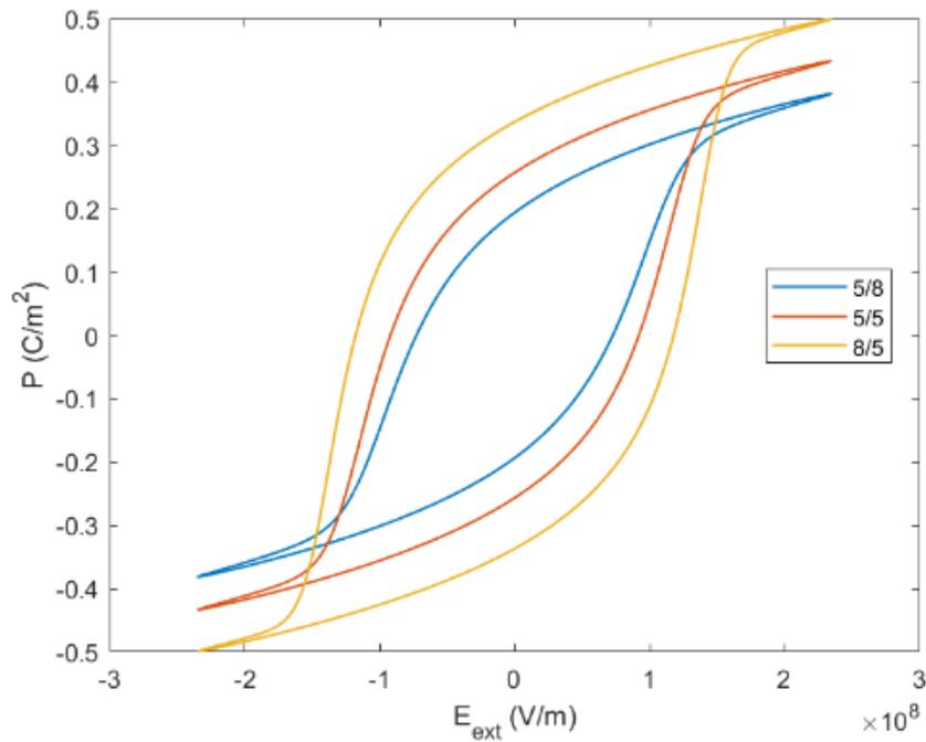
FIGURE 3. Polarization-applied electric field ( $P - E_{ext}$ ) hysteresis loops of PT/ST superlattices with  $\lambda_0 = \xi_0$  at  $T = 298\text{K}$ .
