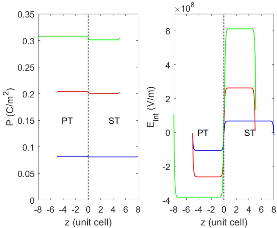
**FIGURE 2.** The profiles of polarization and internal electric field of PT/ST superlattices with  $\lambda_0 = \xi_0$  at  $T = 298\text{K}$ . The thickness ratio  $d_{PT}/d_{ST}$ :  $5u.c/8u.c$  (blue line),  $5u.c/5u.c$  (red line),  $8u.c/5u.c$  (green line).
