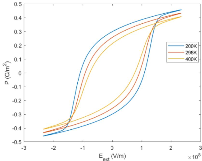
**FIGURE 5.** Polarization-applied electric field ( $P - E_{ext}$ ) hysteresis loops of PT/ST superlattices with  $\lambda_0 = \xi_0$  for thickness ratio  $d_{PT}/d_{ST} = 5/5$ .
