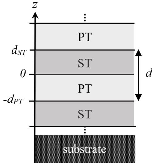
**FIGURE 1.** Schematic illustration of a periodic PT/ST superlattices on a ST substrate. The thickness of PT layer and ST layer are  $d_{PT}$  and  $d_{ST}$ .
