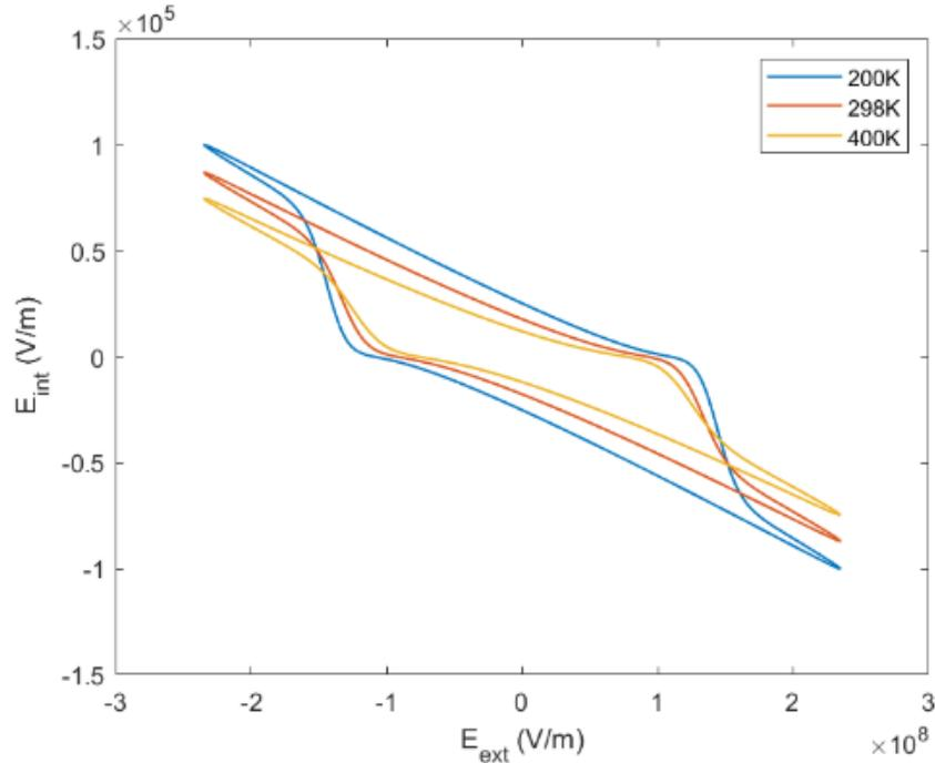
**FIGURE 6.** Internal electric field-applied electric field ( $P - E_{ext}$ ) hysteresis loops of PT/ST superlattices with  $\lambda_0 = \xi_0$  for thickness ratio  $d_{PT}/d_{ST} = 5/5$ .
