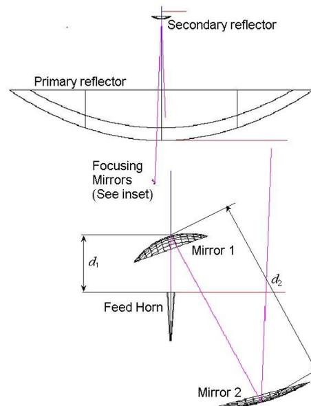
**FIG. 1.** Optical system of a Cassegrain antenna comprising the primary and secondary reflectors and the feed optics.
