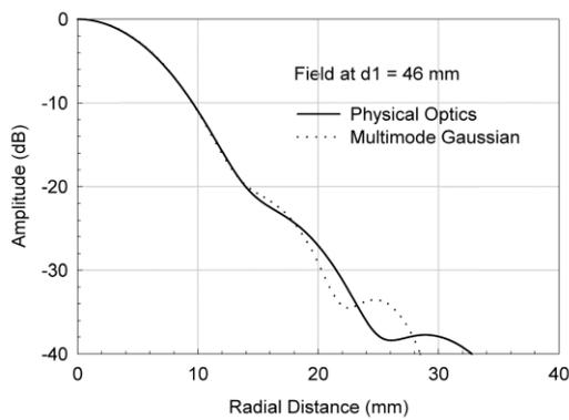
**FIG. 3.** Field of ideal corrugated horn at  $d_1 = 46$  mm from its aperture, frequency 243 GHz.
