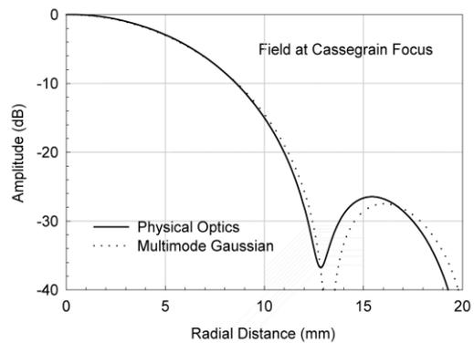
**FIG. 4.** Field at Cassegrain focus plane,  $d_3 = 230$  mm from mirror 2, frequency 243 GHz.
