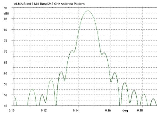
**FIG. 6.** Antenna radiation pattern on antenna axis coordinates showing the offset of the beam.
