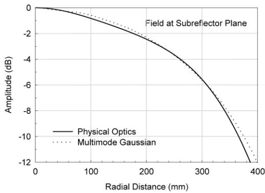
**FIG. 5.** Beam profile at the subreflector at mid-band frequency (243 GHz).
