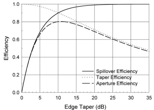
**FIG. 2.** Aperture efficiency for a Cassegrain antenna with fractional blockage  $f_b = 375/6000$  as a function of edge taper.
