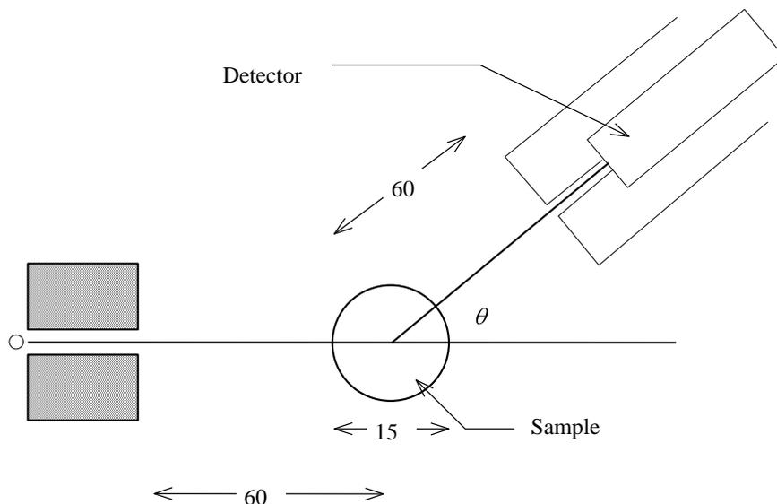
FIG. 2. Arrangement of the apparatus used for the Compton scattering experiments. All dimensions are in mm.
