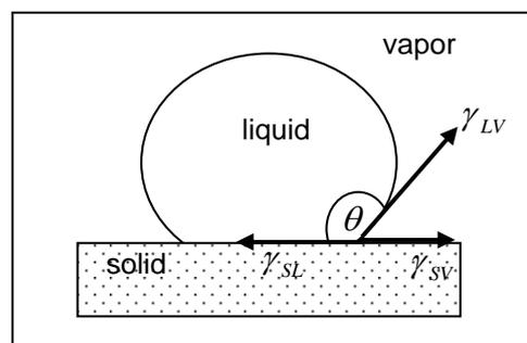
FIG. 2. Schematic diagram of contact angle, showing the balance of surface tension forces.
