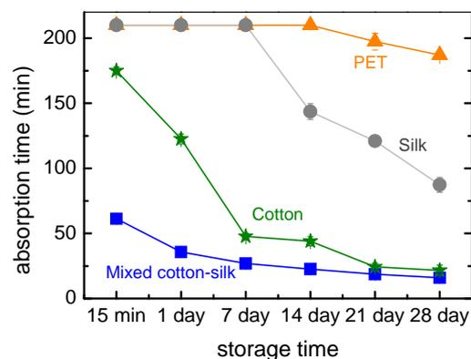
**FIG. 7.** Water droplet absorption time on PET, cotton, silk and mixed cotton-silk, treated for 1 min at pressure of 0.05 torr and RF power of 25 watts, measured at different times after treatment.
