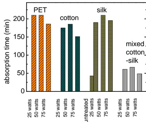
**FIG. 6.** Water droplet absorption time on PET, cotton, silk and mixed cotton-silk as a function of RF power. Plasma pressure and treatment time are 0.05 torr and 1 min, respectively.
