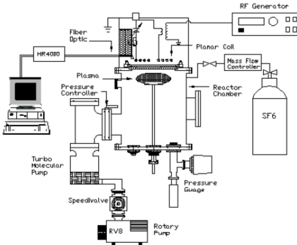
FIG. 1. Schematic diagram of the RF-ICP system.
