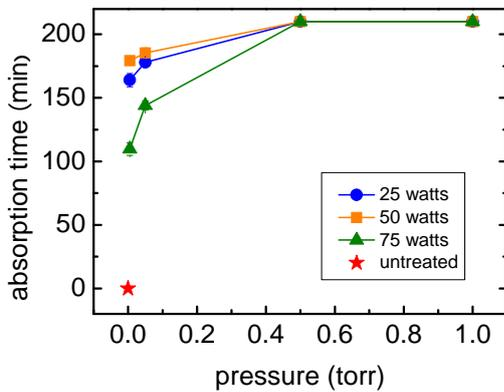
**FIG. 4.** Water droplet absorption time on cotton which were treated for 1 min at different pressures and RF powers. Untreated cotton absorbed water rapidly
