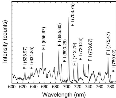
**FIG. 8.** OES spectrum of SF<sub>6</sub> plasma at the pressure of 0.05 torr and the RF power of 25 watts. The spectrum was identified using the NIST atomic wavelength table which indicated F I peaks in the spectrum.
