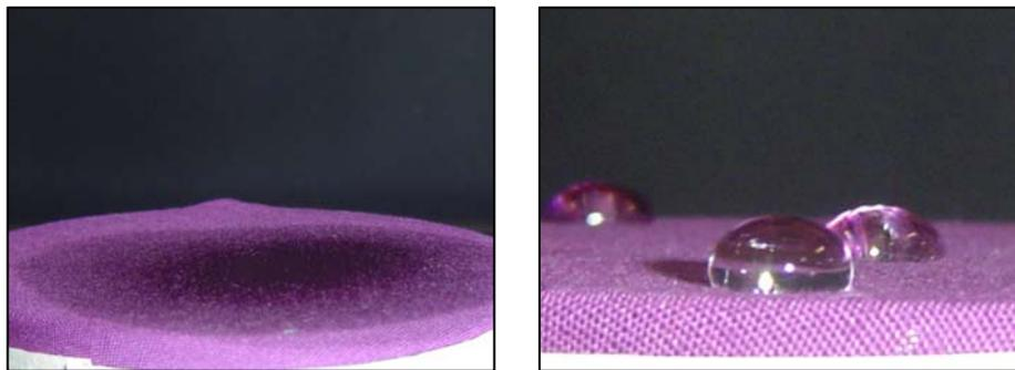
**FIG. 3.** The PET sample (a) before and (b) after the SF<sub>6</sub> plasma treatment. The water droplet is instantly absorbed into the untreated fabric while stay unabsorbed on the treated fabric surface.
