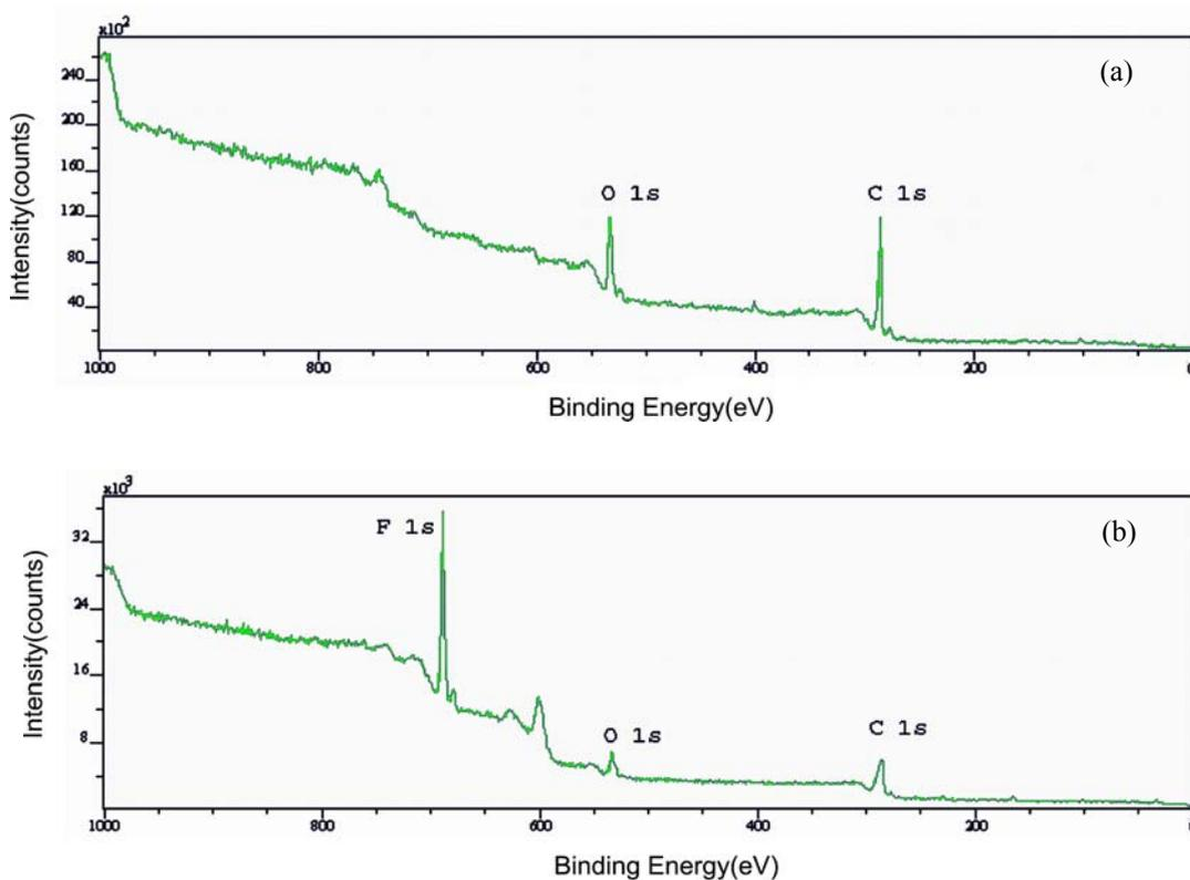
**FIG. 9.** Survey scans of XPS on silk samples; (a) untreated, and (b) treated sample. The treated sample was exposed to SF<sub>6</sub> plasma for 1 min at the pressure of 0.5 torr and the RF power of 50 watts.
