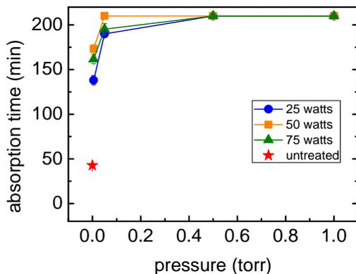
**FIG. 5.** Water droplet absorption time on silk which were treated for 1 min at different pressures and RF powers.
