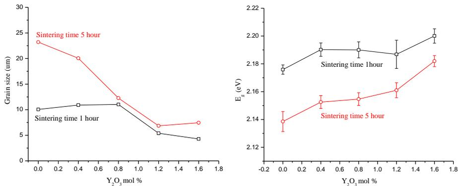
FIG. 2. Grain size (left) and Energy band gap dependence on the doping level of  $Y_2O_3$  for 1 and 5 hours sintering time.
