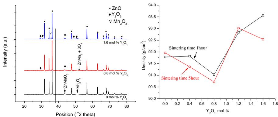
**FIG. 1.** XRD pattern for 5 hours sintering time (left) and the variation of density with the mol% of Y<sub>2</sub>O<sub>3</sub> for 1 and 5 hours sintering time (right).
