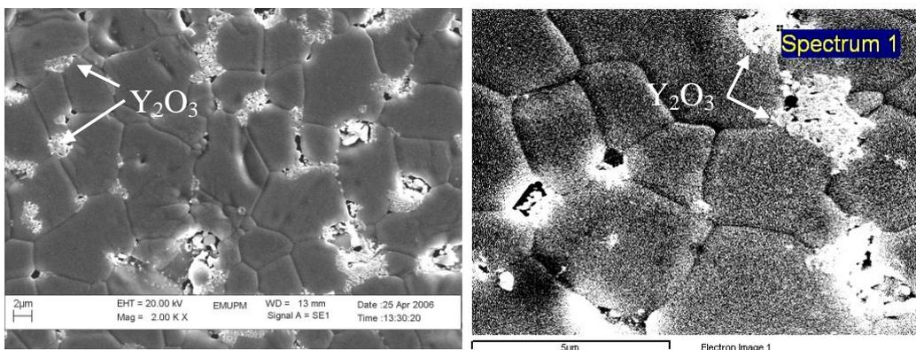
FIG. 3. SEM micrograph showing elemental distribution at different areas for 5 h at 1.6 mol%.
