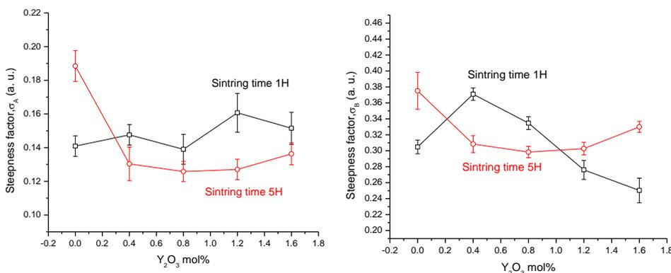
FIG. 4. Dependence of the steepness factor  $\sigma_A$  (left),  $\sigma_B$  (right) on  $Y_2O_3$  mol%.
