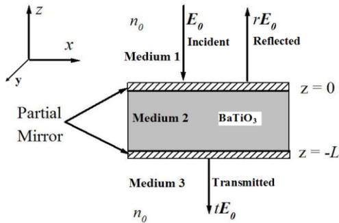
FIG. 1. Geometry of the Fabry-Perot interferometer system.
