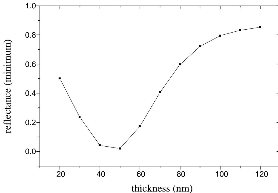
**FIG. 8.** The relationship between the minimum reflectivity with the thickness of layer.
