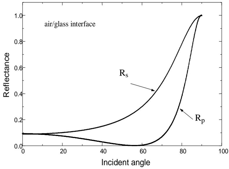
FIG. 2. The reflectance for the P and S polarization as a function of incidence angles for air/glass interface.
