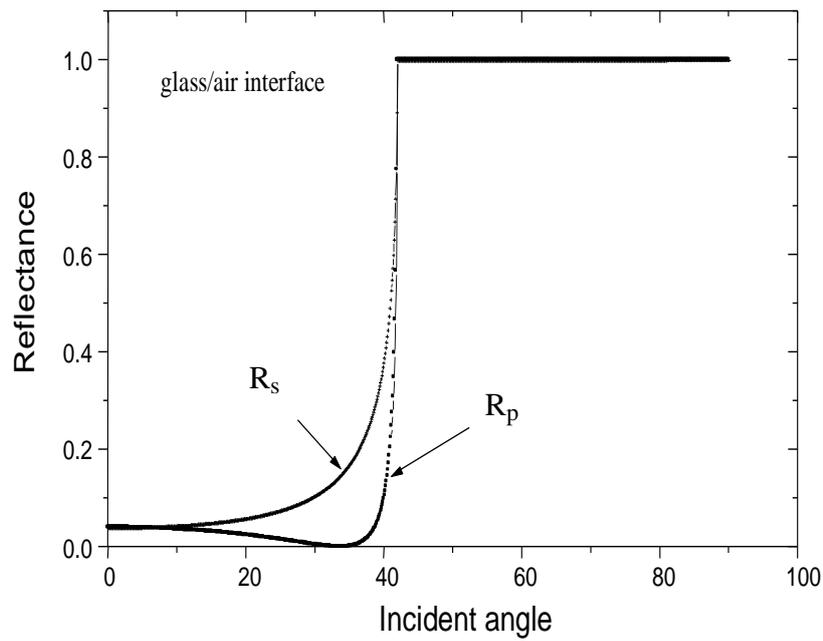
FIG. 4. The reflectance for the P and S polarization as a function of incidence angles for glass/air interface.
