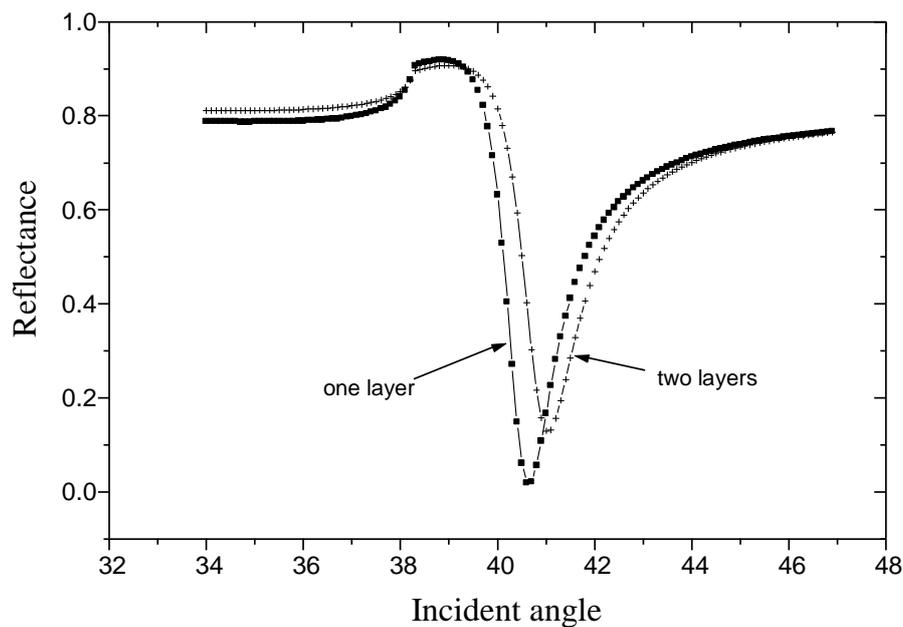
FIG. 11. Reflectivity curves for one layer and two layer of gold thin film as a function of incident angle.
