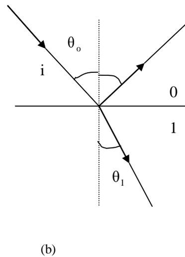
**FIG. 1.** (a) Propagation of EM fields in multilayer thin film system with  $N-1$  layers, and (b) an incident ray  $I$  hits interface 0-1 at an angle  $\theta_0$  and refracted into medium 1 at angle  $\theta_1$  and reflected in medium 0 at angle  $\theta_0$ .
