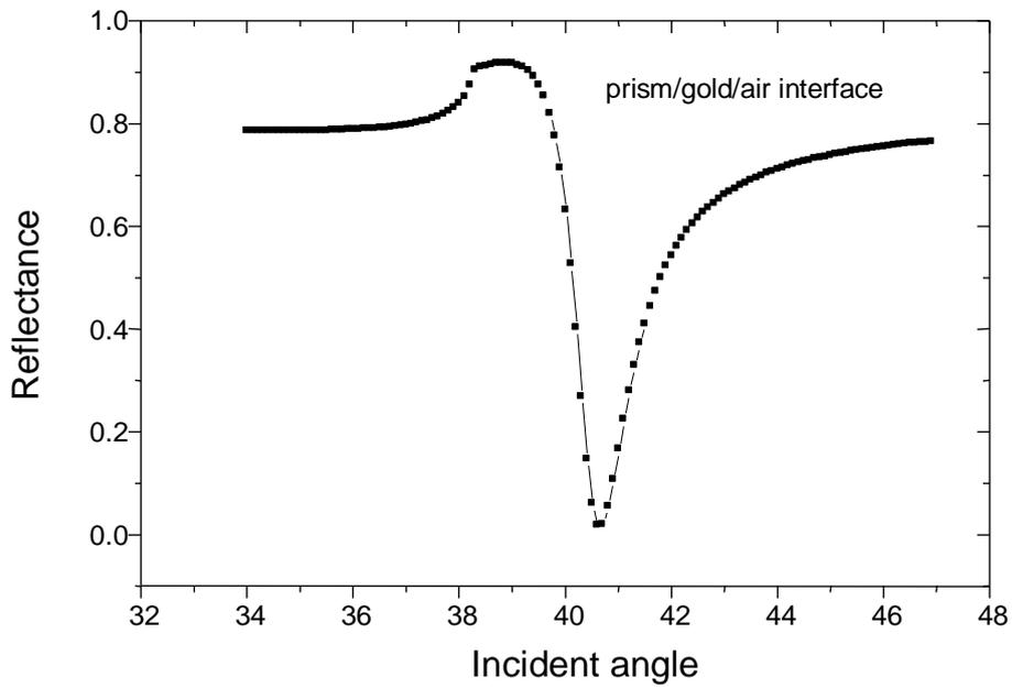
FIG. 5. The reflectance for the p-polarized light as a function of incidence angles for prism/gold/air interface.
