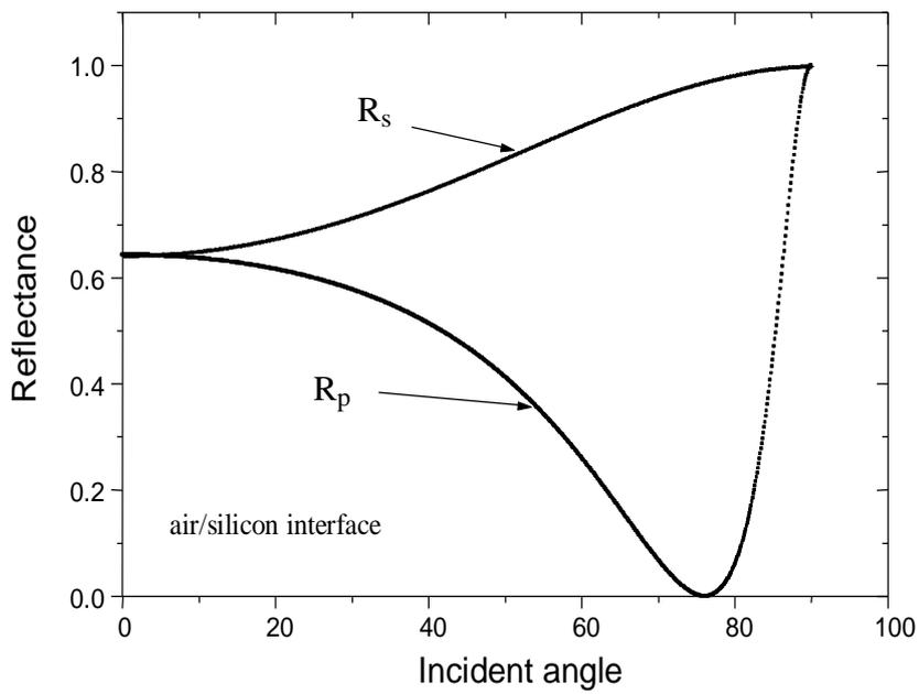
FIG. 3. The reflectance for the P and S polarization as a function of incidence angles for air/silicon interface.
