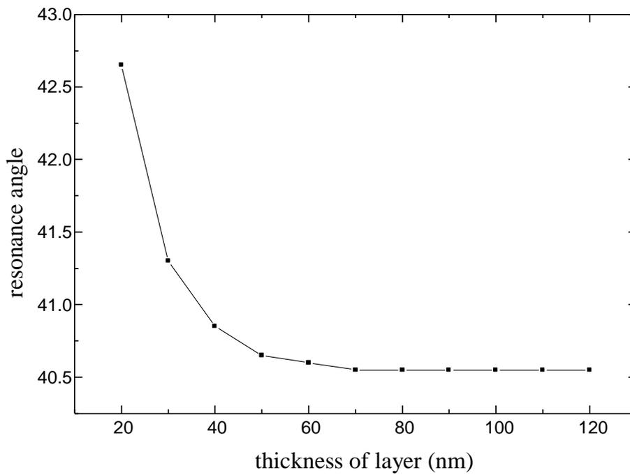
FIG. 7. The relationship between the resonant angle,  $\theta_{spr}$  with the thickness of layer.
