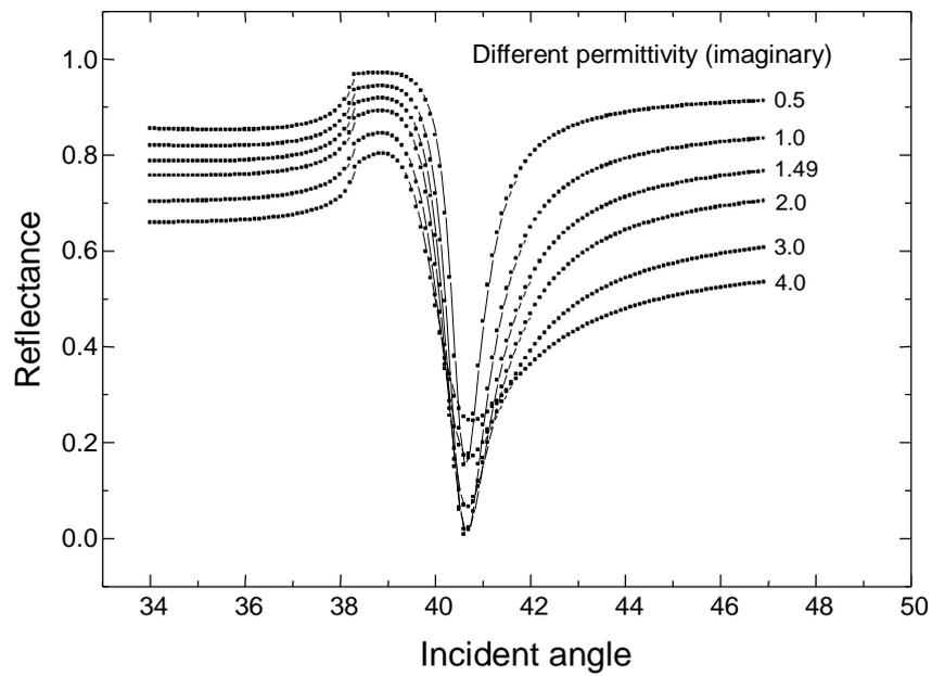
FIG. 10. The plot of reflectance as a function of incidence angle for different permittivity (imaginary).
