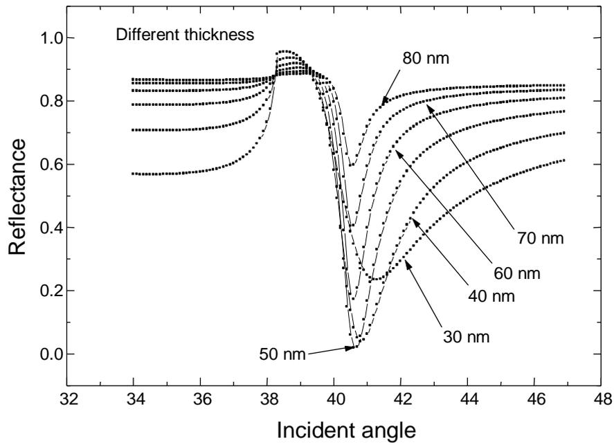
FIG. 6. The plot of reflectance as a function of incidence angle for different thickness.
