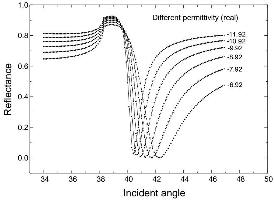
FIG. 9. The plot of reflectance as a function of incidence angle for different permittivity (real).
