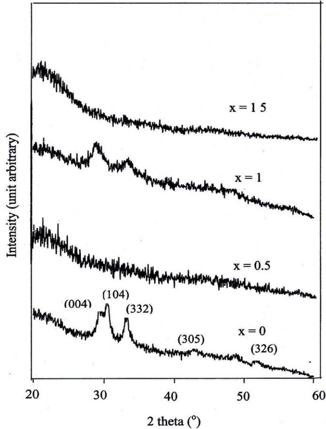
FIG. 2. The XRD spectra for all films annealed at 700°C for 2 hours.
