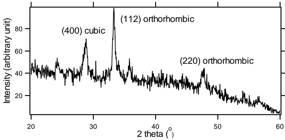
FIG. 3. The XRD spectrum for the film x = 1.5 annealed at 800°C for 2 hours.
