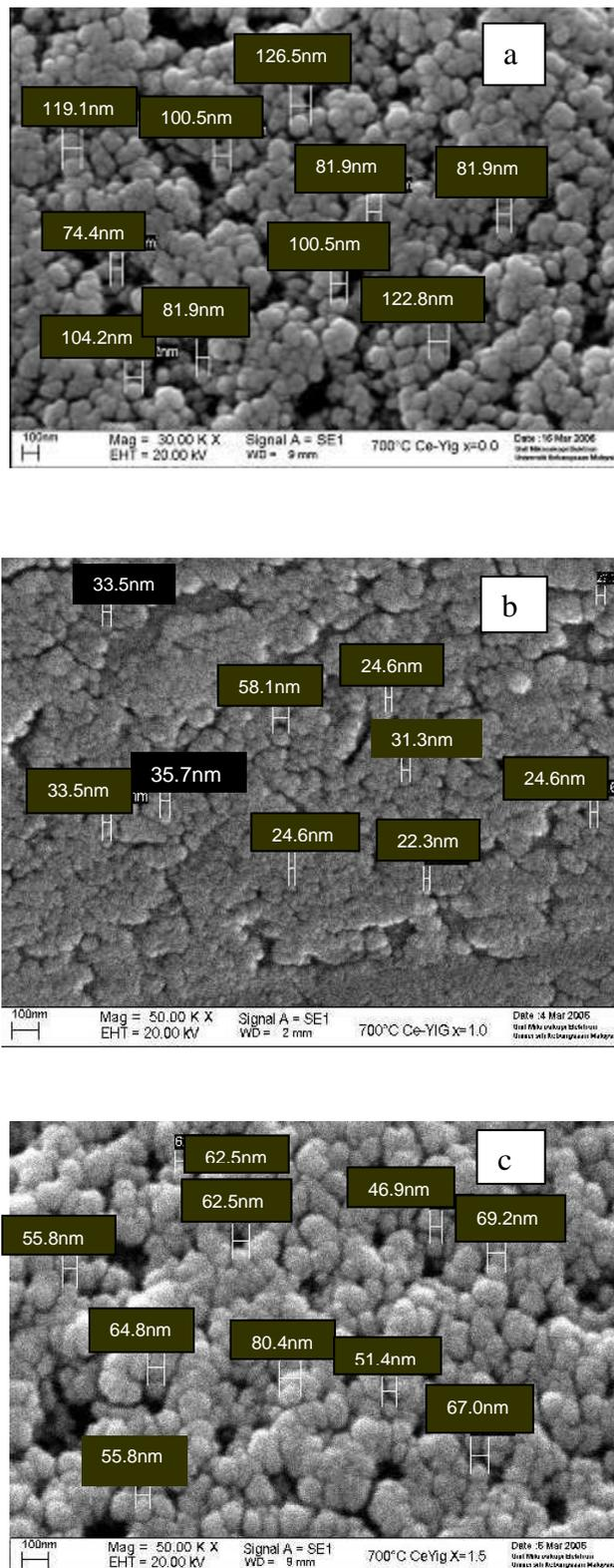
**FIG. 5.** SEM micrographs of the films (a)  $x = 0$  (b)  $x = 1$  and (c)  $x = 1.5$ .
