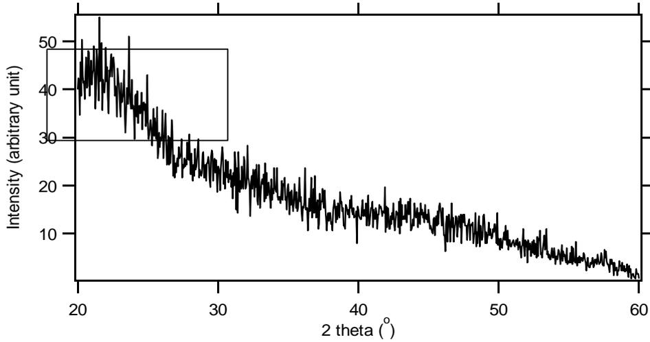
FIG. 1. The typical XRD spectrum for the as-prepared films.
