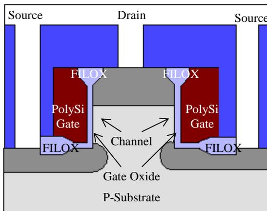
**FIG. 1.** Schematic structure of vertical double gate MOSFET (VDGM).
