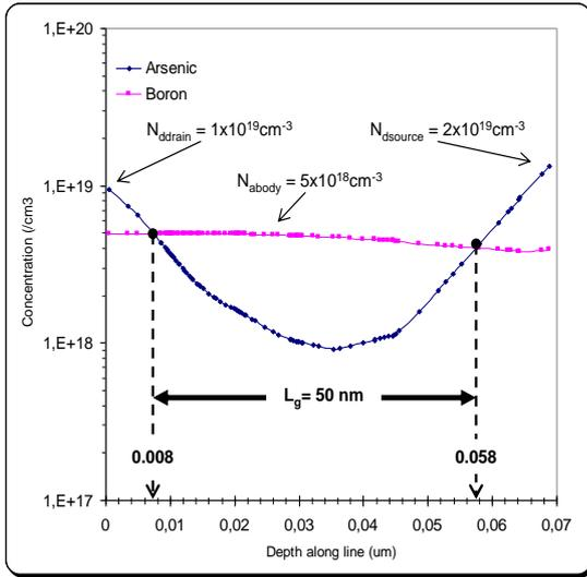
**FIG. 2.** Vertical doping profiles of design VDGM with  $L_g = 50$  nm, drain doping,  $N_{ddrain} = 1 \times 10^{19} \text{ cm}^{-3}$ , source doping,  $N_{dsouce} = 2 \times 10^{19} \text{ cm}^{-3}$  and body doping,  $N_{abody} = 5 \times 10^{18} \text{ cm}^{-3}$ .
