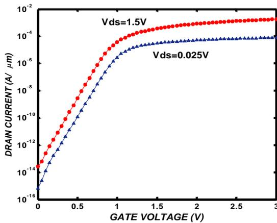
**FIG. 4.** Transfer characteristic of VDGM device with  $L_g = 50$  nm,  $T_{OX} = 3$  nm,  $N_{abody} = 5 \times 10^{18}$  cm<sup>-3</sup>;  $V_S = V_B = 0$  V.
