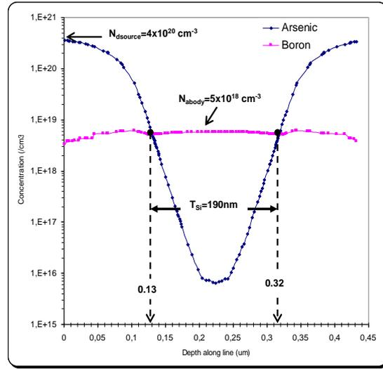
**FIG. 3.** Horizontal doping profiles of design VDGM with silicon thickness  $t_{si} = 190$  nm, drain doping,  $N_{ddrain} = 4 \times 10^{20} \text{ cm}^{-3}$ , source doping,  $N_{dsouce} = 4 \times 10^{20} \text{ cm}^{-3}$  and body doping,  $N_{abody} = 5 \times 10^{18} \text{ cm}^{-3}$ .
