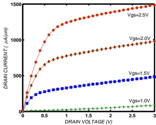
**FIG. 5.** Output characteristic of VDGM with  $L_g = 50$  nm,  $T_{OX} = 3$  nm,  $N_A = 5 \times 10^{18}$  cm<sup>-3</sup> for  $V_{GS} = 1, 1.5, 2$  and 2.5 V.
