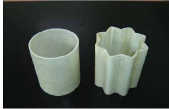
**FIG. 2.** Cylindrical and radial corrugated specimens (CCT3, and RCCT).
