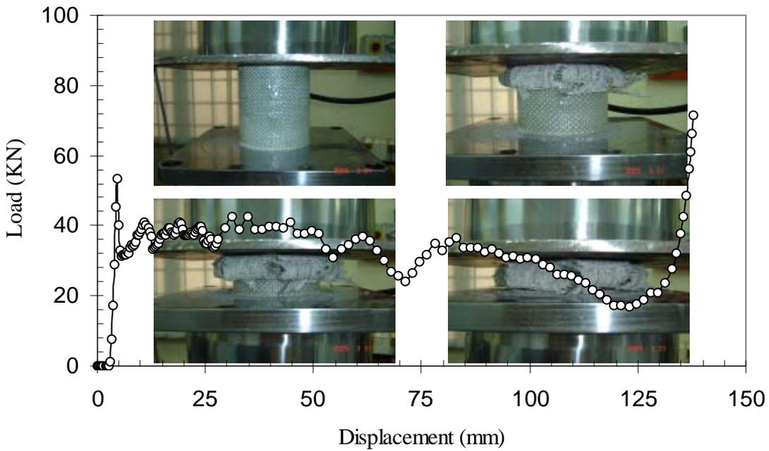
FIG. 5. Load-displacement curve and deformation history of CCT3.
