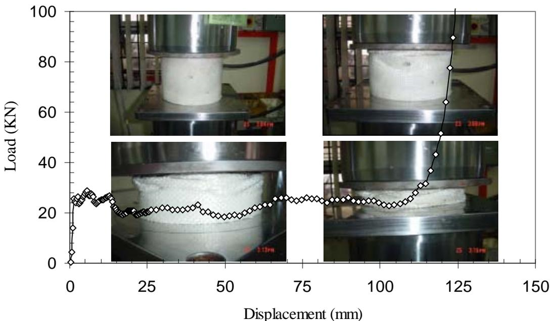
**FIG. 3.** Load-displacement curve and deformation history of CCT1.
