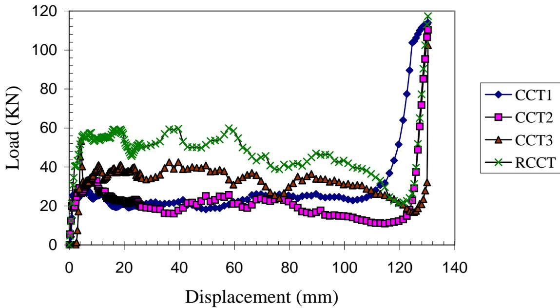
FIG. 7. Load-displacement curve of CCT1, CCT2, CCT3, and RCCT.
