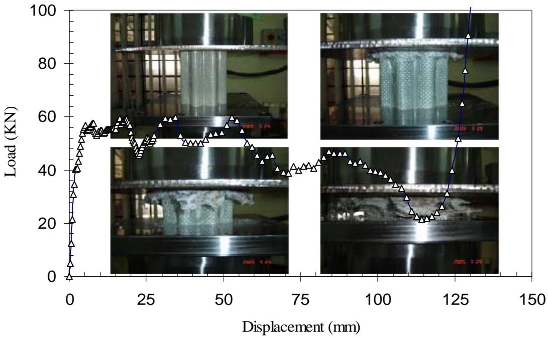
FIG. 6. Load-displacement curve and deformation history of RCCT.
