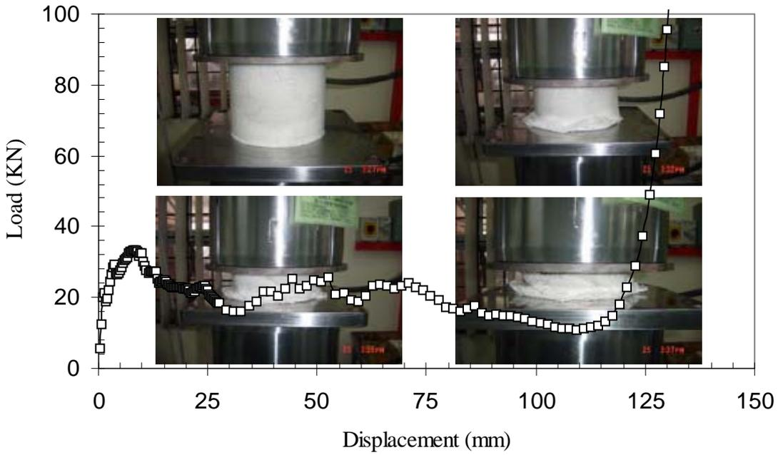
FIG. 4. Load-displacement curve and deformation history of CCT2.
