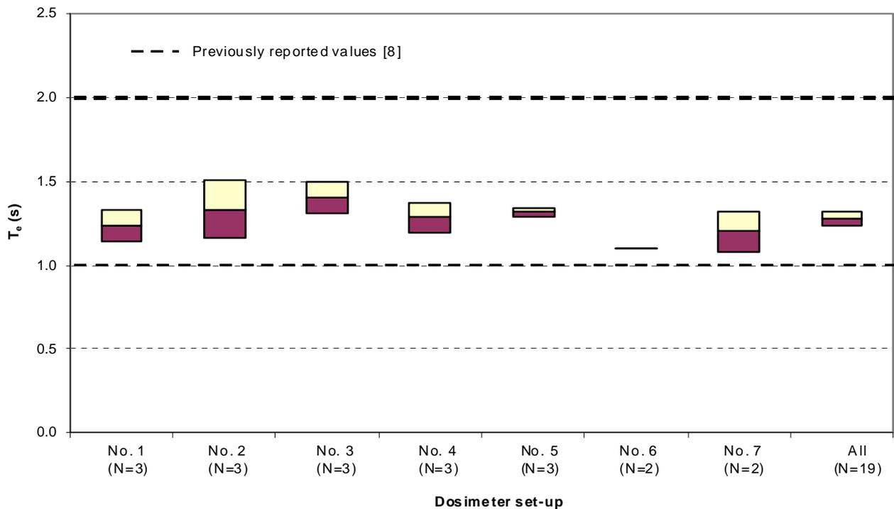
**FIG. 2.** Experimentally obtained timer error  $T_e$  with standard uncertainty, for a Co-60 teletherapy unit in comparison with the previously reported values.
