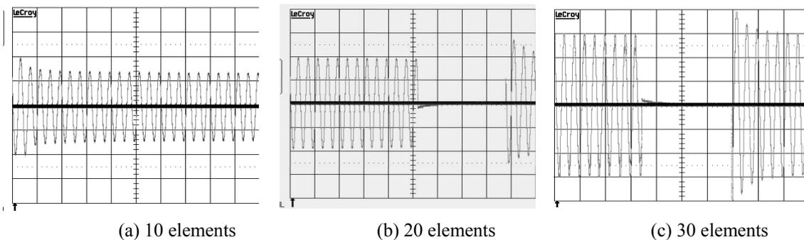
**FIG. 2.** Limiting behavior of fault current limiter for (a) 10 Bi-2212 elements connected in series, (b) 20 Bi-2212 elements connected in series, and (c) 30 Bi-2212 elements connected in series.
