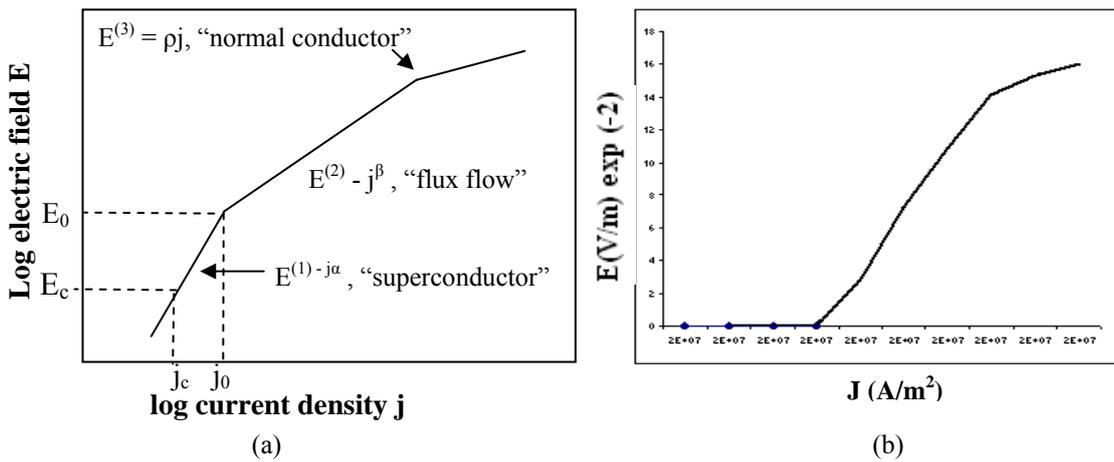
**FIG. 1.** (a) Current-voltage characteristic of high-temperature superconductor (HTS) materials, (b)  $E(j)$  for Bi2212 superconductor elements.
