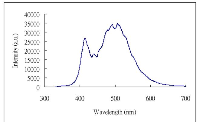
**FIG. 3.** Photoluminescence spectrum of F8P on ITO/glass.
