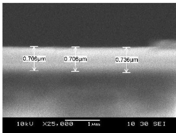
FIG. 1. SEM cross section of the F8P/ITO/glass.
