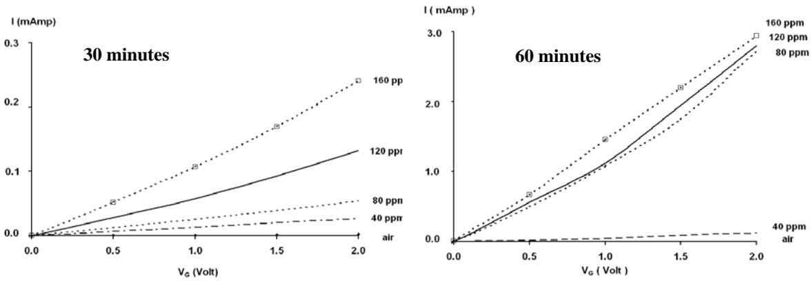
**FIG. 2.** The forward current–voltage characteristic of ZnO gas sensor oxidized at 30 minutes and 60 minutes for different H<sub>2</sub> concentration. The operating temperature is 400°C.
