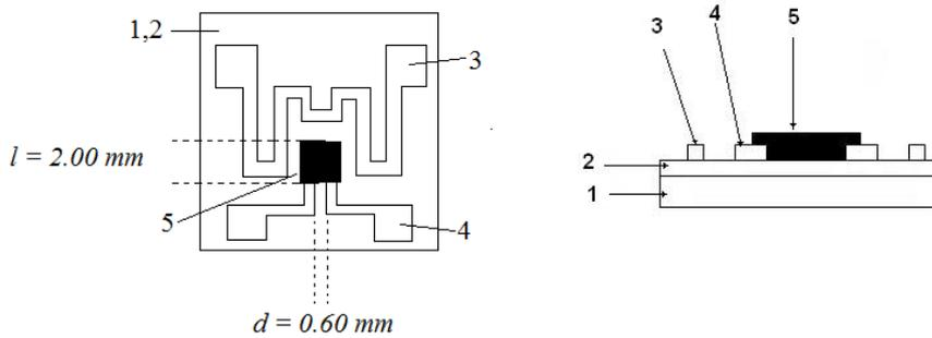
**FIG. 1.** The schematic cross section and top view of the prepared gas sensor; 1- Si substrate, 2- SiO<sub>2</sub> layer, 3- Ti/Pt heating element, 4- Ti/Pt electrodes and 5- ZnO thin film.
