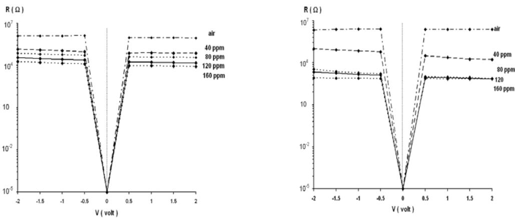
**FIG. 4.** The R-V characteristic of the ZnO gas sensor for (a) 30 minutes and (b) 60 minutes samples.
