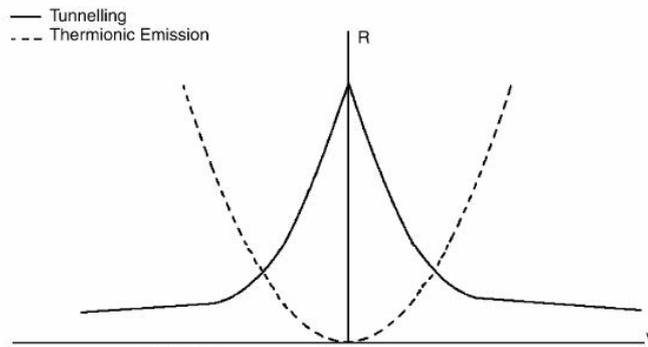
**FIG. 3.** Theoretical R-V characteristics associated with thermionic emission and tunneling [5].
