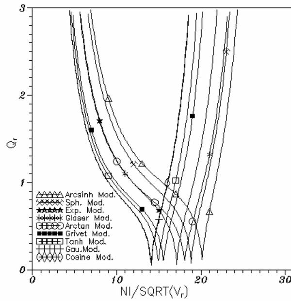
FIG. 4. The radial distortion parameter  $Q_r$ , as a function of the excitation parameter  $NI/\sqrt{V_r}$  for each distributions.
