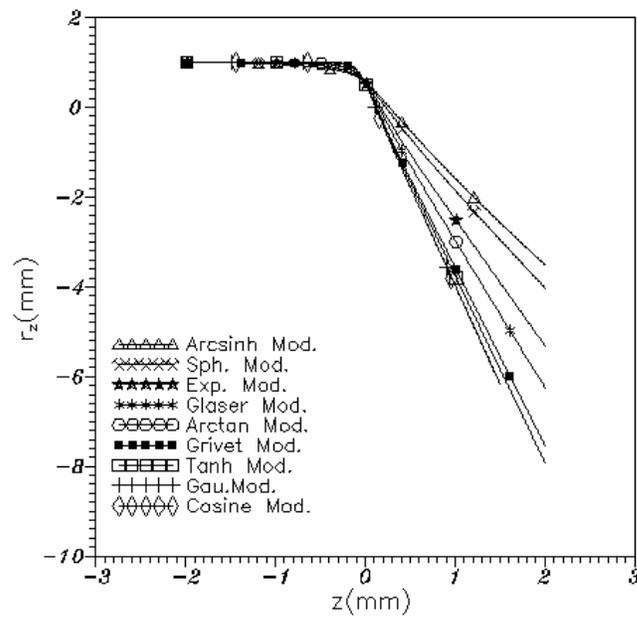
FIG. 3. The electron trajectory along the optical interval  $-3 \leq z \leq 3$  for each model at  $(f_p)_{\min}$ .
