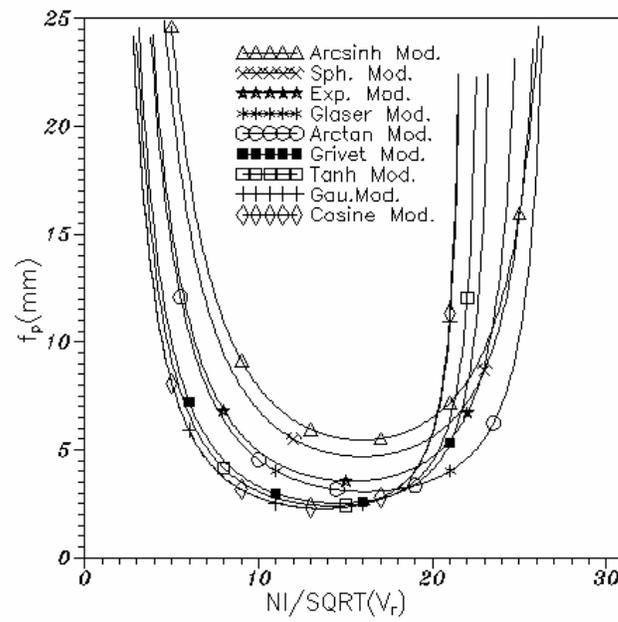
FIG. 2. The variation of the projector focal length  $f_p$  versus the excitation parameter  $NI/\sqrt{V_r}$  for each distribution.
