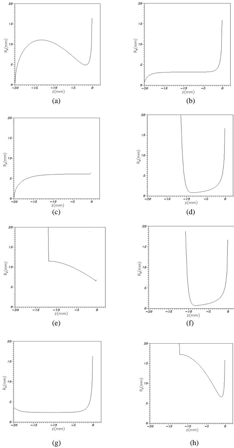
**FIG. 7.** The polepieces shape for: (a) Glaser's bell-model (Inverse tangent model); (b) Grivet-Lenez model; (c) Exponential field model; (d) Gaussian field model; (e) Spherical polepiece model; (f) Cosine field model; (g) Hyperbolic tangent model; (h) Inverse hyperbolic sine model.
