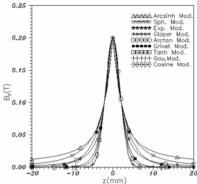
FIG. 1. The axial magnetic field distribution for various models at ( $B_0 = 0.2T$ ,  $a = 4.230$  mm,  $L = 40$  mm).
