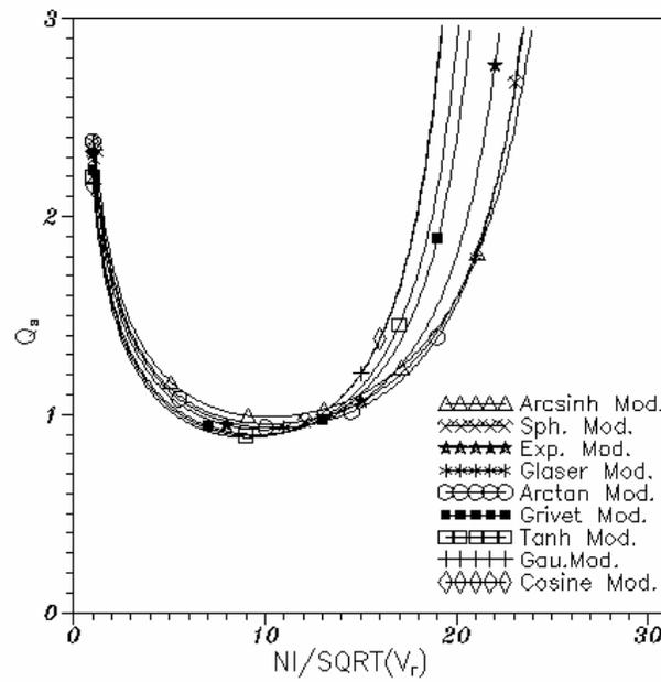
FIG. 5. The spiral distortion parameter  $Q_s$ , as a function of the excitation parameter  $NI/\sqrt{V_r}$  for each distributions.
