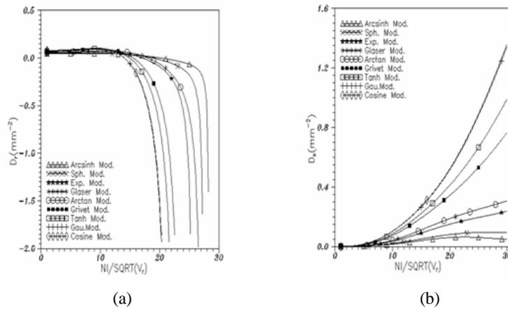
**FIG. 6.** The variation of the: (a) radial distortion coefficient  $D_r$ , and (b) spiral distortion coefficient as a function of the excitation parameter  $NI/\sqrt{V_r}$  for each distributions.
