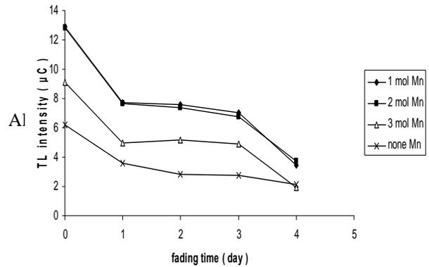
FIG. 5. Fading rate of ~250°C TL peak at room temperature of nanophosphors with different Mn concentration.
