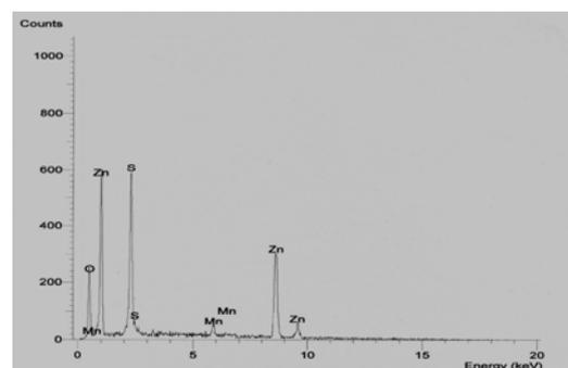
FIG. 2. Elemental composition of the nanophosphors.
