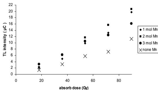
FIG. 4. TL sensitivity of nanophosphors with different Mn molarity.
