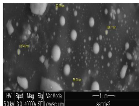
FIG. 1. Micrograph of ZnS:Mn nanophosphors.
