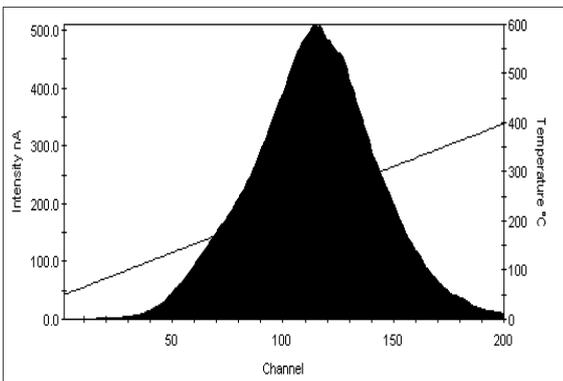
FIG. 3. Typical TL glow curve of ZnS:Mn nanophosphors.
