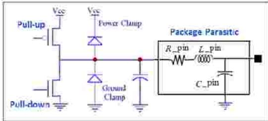
FIG. 1. Schematic of IBIS output buffer model.
