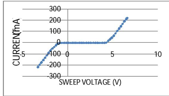
FIG. 6. Pull-down I/V curve.
