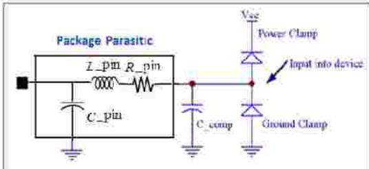
FIG. 2. Schematic of IBIS input buffer model.
