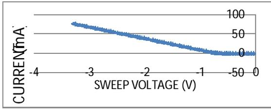
FIG. 3. Power clamp I/V curve referenced to  $V_{CC}$ .
