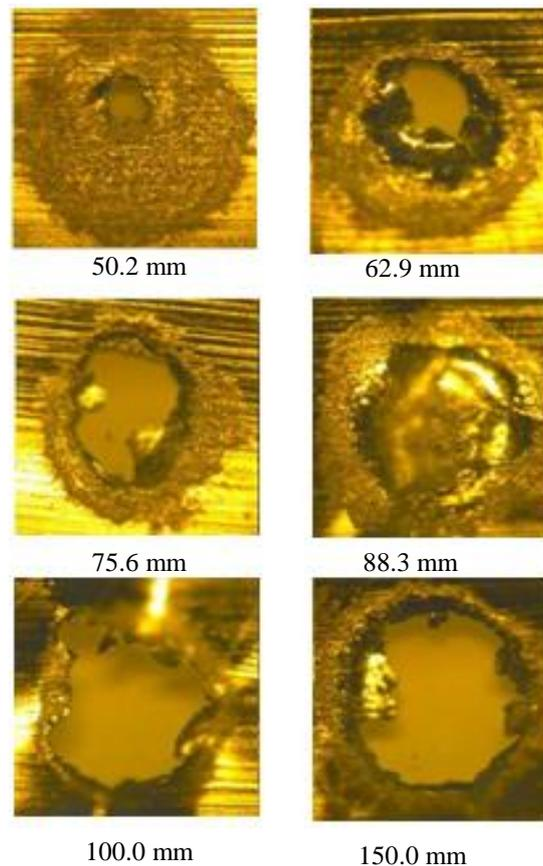
Fig. 3 Images of laser plasma interaction with aluminum target.
