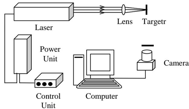
Fig. 2 Experimental setup of IR laser plasma interaction with aluminum target.
