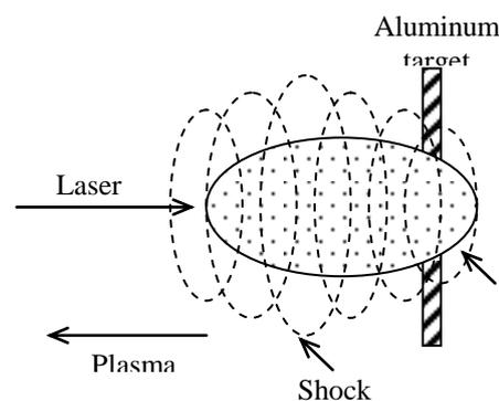
Fig. 7 Plasma generation associated with shock waves impinges on aluminum.
