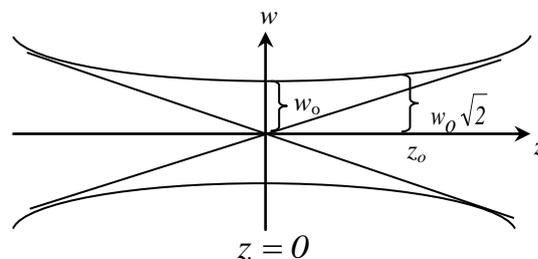
Fig. 1 Laser beam in the form of Gaussian beam after been focused by lens. At a focal point,  $z = 0$ , the beam waist is  $w_o$  and at Rayleigh region  $z_o$  the beam waist is extend to  $w_o \sqrt{2}$ .
