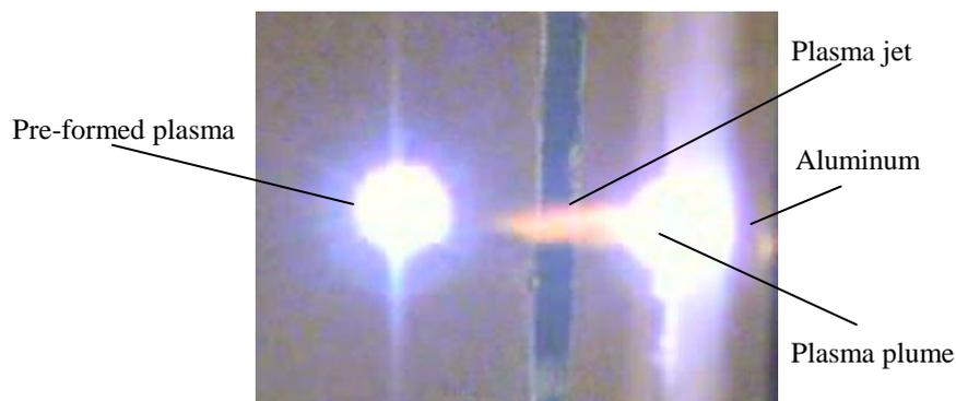
Fig. 4 Pre-formed plasma, plasma jet and aluminum plasma plume during interaction with aluminum target.
