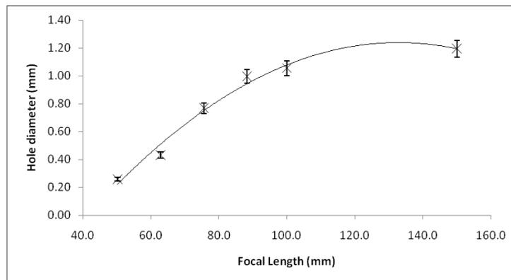
Fig. 5 Hole size on aluminum target as a function of lens focal length.
