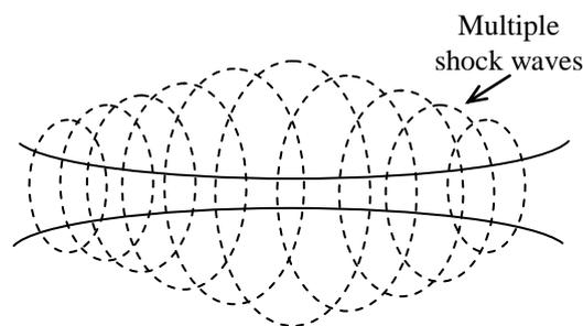
Fig. 6 Multiple shock waves induced when the pulsed laser beam is brought by a lens.
