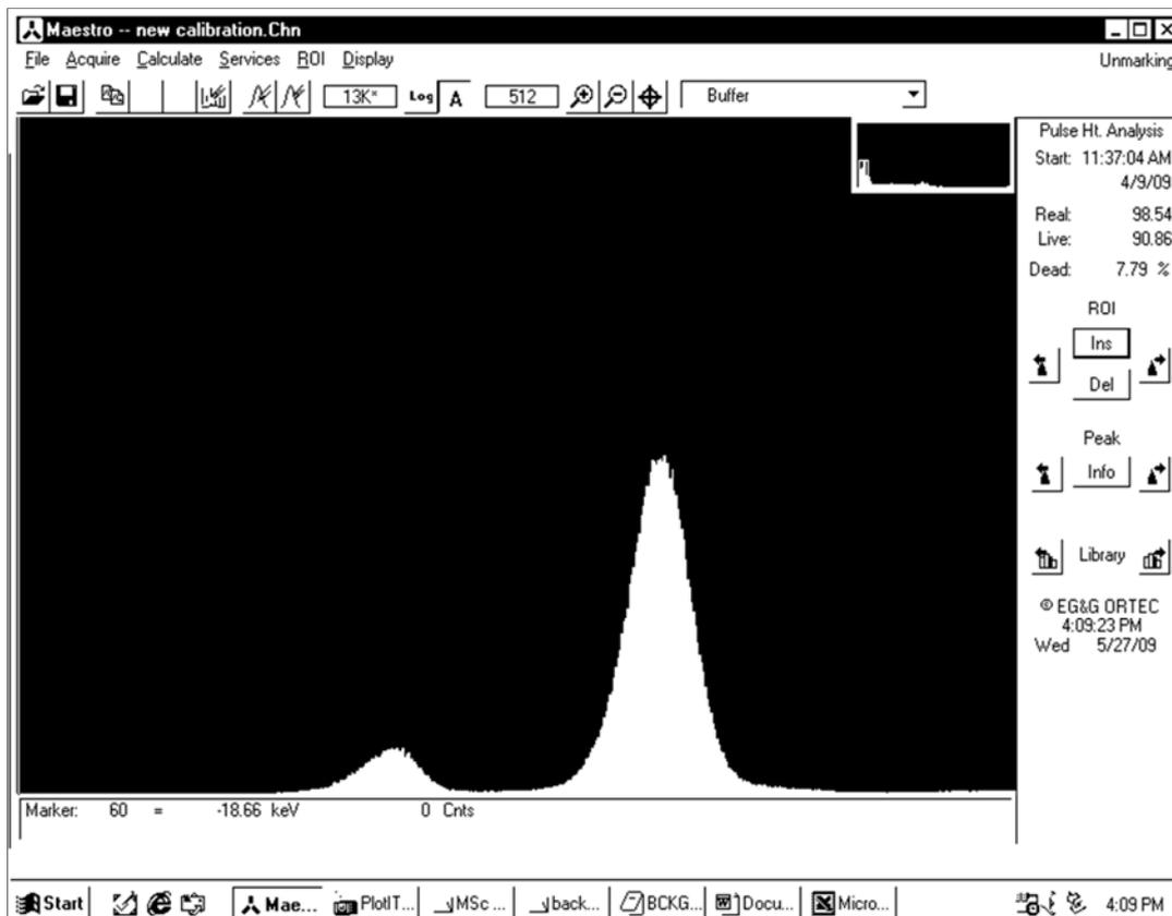
Fig. 2: Spectrum of Am-241 detected by our NaI(Tl) detector.
