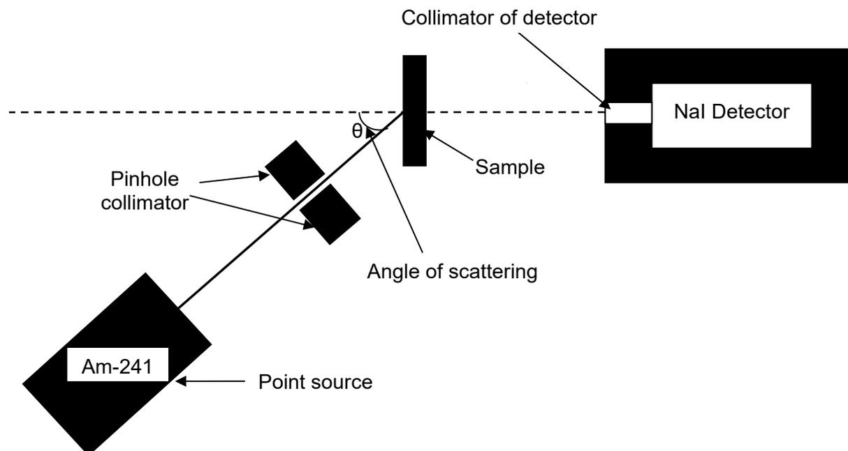
Fig. 1: Experimental set up for scattering study.
