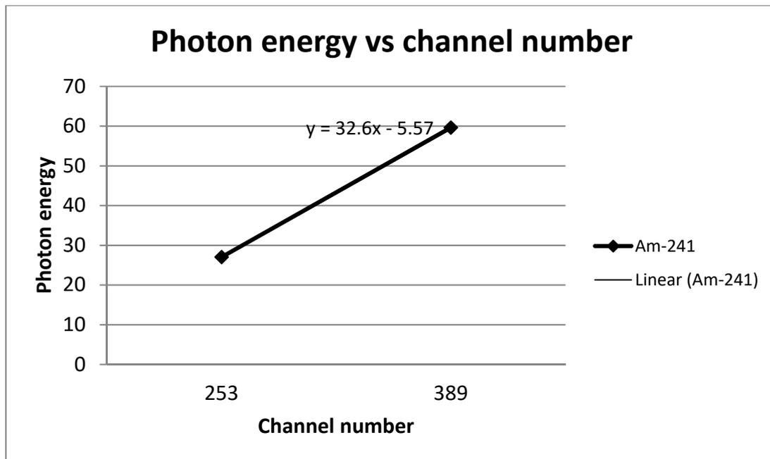
Figure 3: Calibration curve which showing channel number versus photon energy of Am-241.
