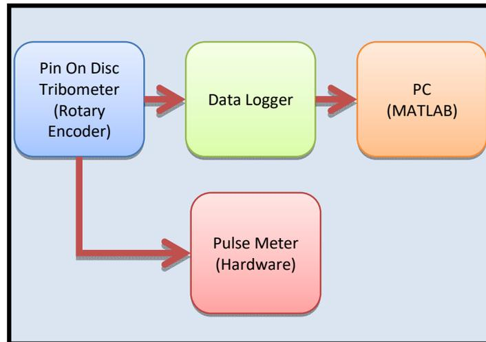
**FIGURE 2.** System Block Diagram
