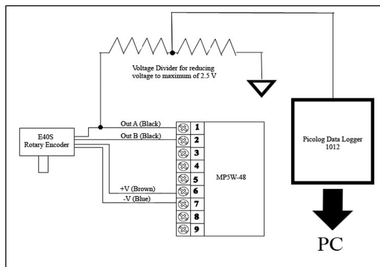
**FIGURE 3.** Circuit diagram of the connection between data logger and pulse meter from the encoder.
