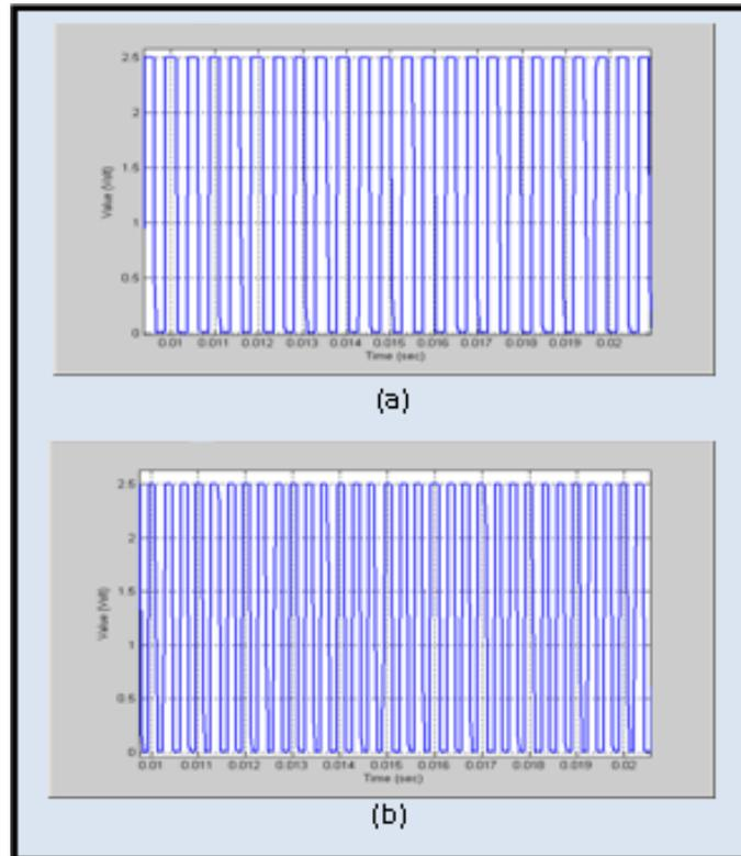
FIGURE 4. Example square wave sample captured by Data logger at (a) 200 RPM and (b) 300 RPM
