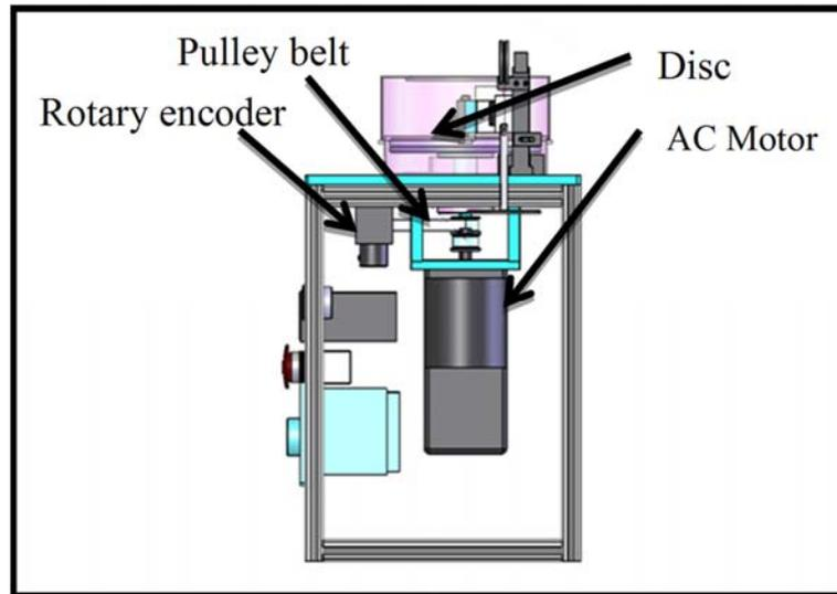
FIGURE 1. Rotary encoder mounted inside POD Tribometer
