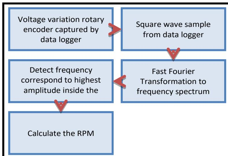
FIGURE 5. Algorithm for finding the RPM
