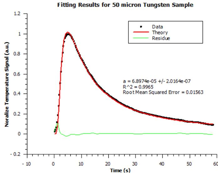
**FIGURE 9:** Fitting Results for W (50 μm Thick) showing thermal diffusivity value
