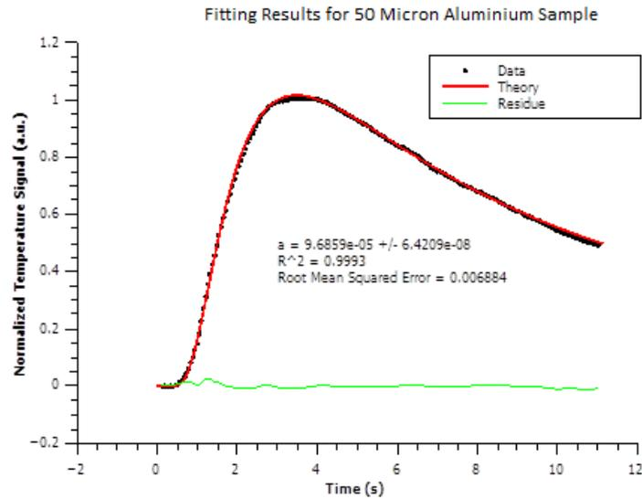
FIGURE 5: Fitting Results for Al (50  $\mu$ m Thick) showing thermal diffusivity value
