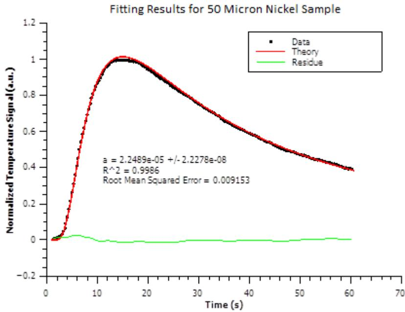
FIGURE 7: Fitting Results for Ni (50 μm Thick) showing thermal diffusivity value
