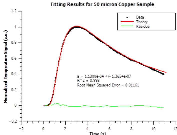
FIGURE 6: Fitting Results for Cu (50  $\mu$ m Thick) showing thermal diffusivity value
