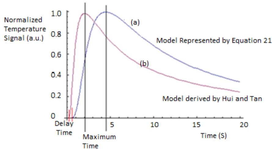
FIGURE 2: Temperature transients for the two curves
