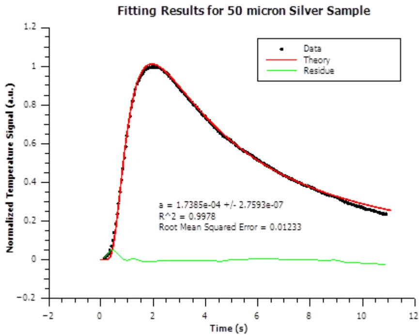
FIGURE 8: Fitting Results for Ag (50 μm Thick) showing thermal diffusivity value
