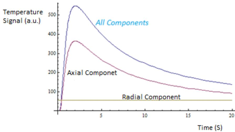
FIGURE 4: Plotted parts of components of the Theoretical Model Derived by Hui and Tan
