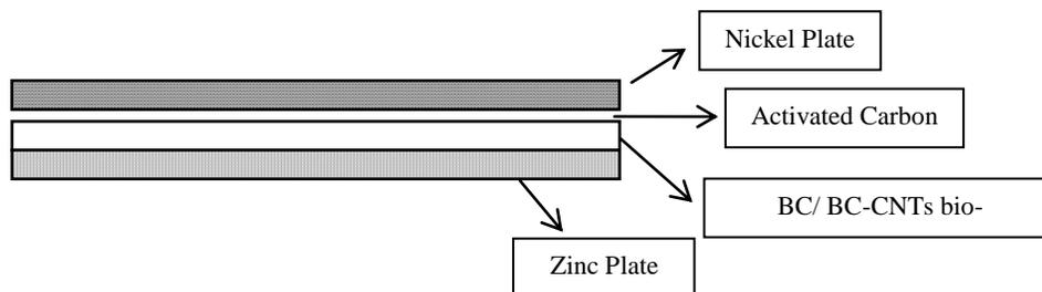
FIGURE 1: Design of Zinc Air Fuel Cell
