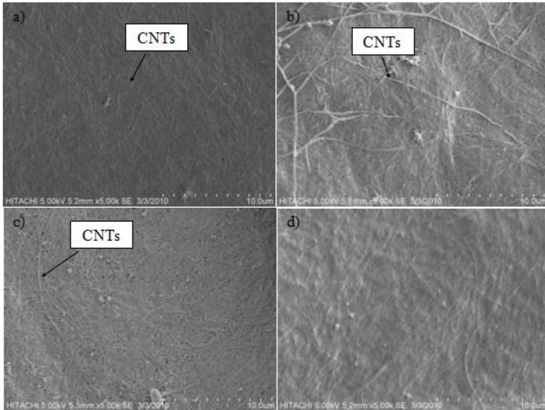
**FIGURE 4::** Morphology of (a) BC7/CNTs2, (b) BC7/CNTs5, (c) BC7/CNTs8, and (d) BC7
