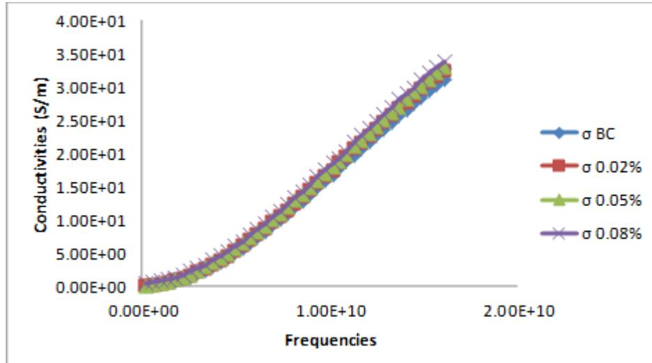
**FIGURE 2:** Conductivities of BC5, BC5-CNTs2 FB-CVD, BC5-CNTs5 FB-CVD, BC5-CNTs8 FB-CVD at Different Frequencies
