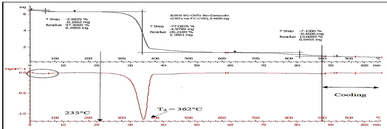
FIGURE 7: Sample TGA result for BC7/CNTs5 FC-CVD
