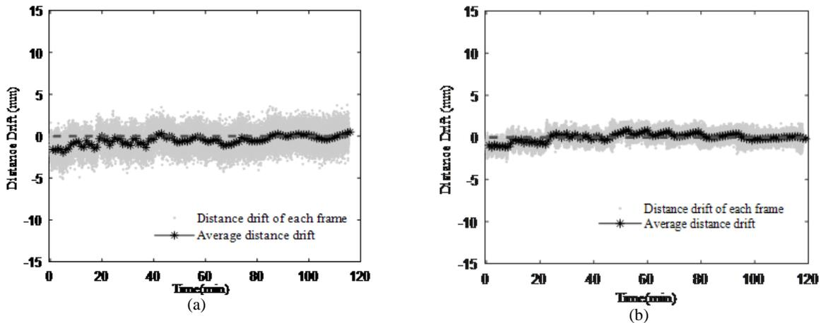
**FIGURE 2.** Distance drift over 120 minutes for (a) Argos<sup>3D</sup> P320 and (b) Argos<sup>3D</sup> P330. The grey dot represents the average of  $9 \times 9$  ROI each frame captured and the black line is referred to the average distance drift per second.
