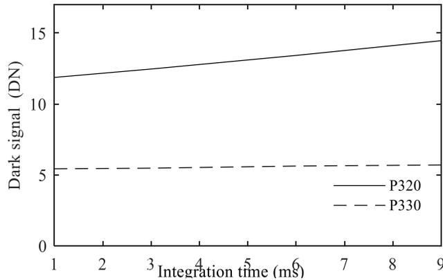
FIGURE 3. Dark signal against integration time plot of Argos<sup>3D</sup> P320 and Argos<sup>3D</sup> P330 ToF camera.
