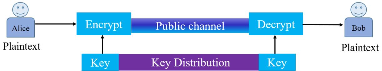
**FIGURE 1.** Structure of Secure Communications. Key is distributed using secure key distribution channel. Then the key is transferred from the key distribution channel to the communication channel at the sender and receiver's sites. Plaintext from sender Alice is encrypted into ciphertext and the ciphertext is transmitted through a public channel to the receiver Bob. Bob decrypts the ciphertext using the key into plaintext.
