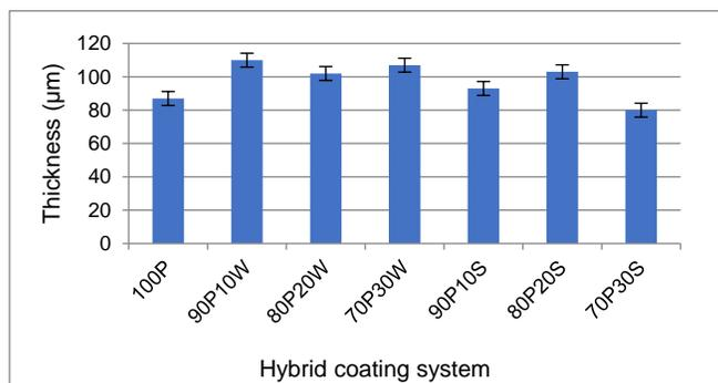
FIGURE 1. Thickness of coating systems developed.
