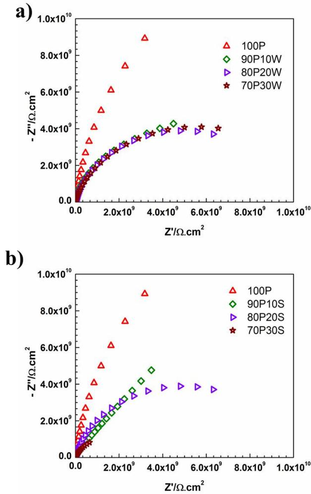
FIGURE 3. Nyquist plot for (a) water-based system and (b) solvent based system after 15 days of immersion
