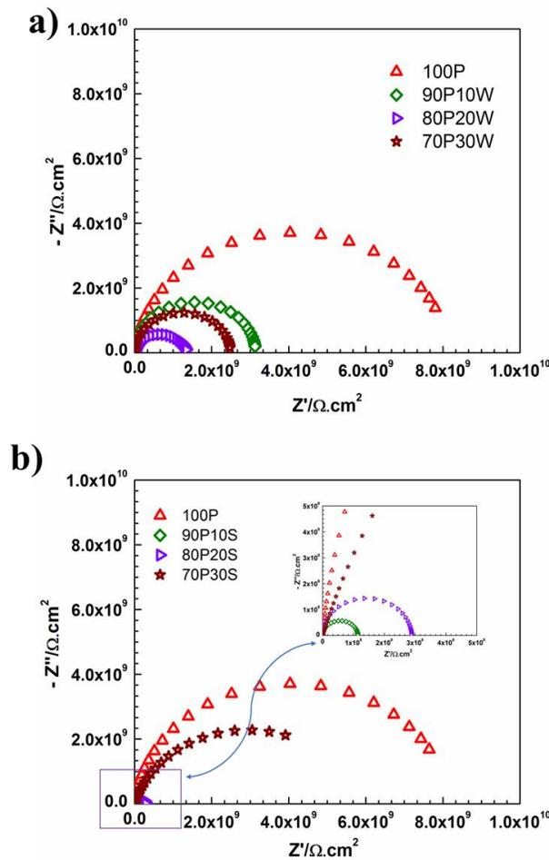
FIGURE 2. Nyquist plot for (a) water-based system and (b) solvent-based system after 1 day of immersion
