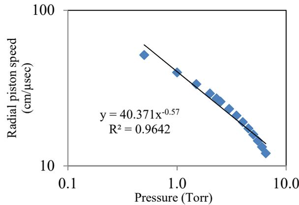
**FIGURE 8.** The variation of computed magnetic piston speed with respect to pressure operating at 38 kV in deuterium for the Imperial College Plasma focus machine
